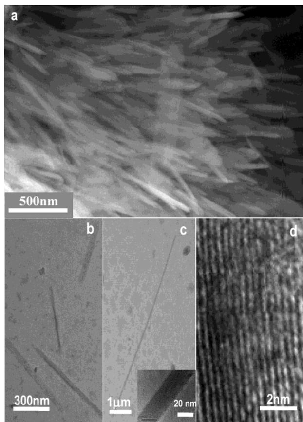
**Figure 2.** SEM and TEM images of Sb nanowires after aging the starting solution for 8 days: (a) FE-TEM image of the synthesized Sb nanowires; (b, c) typical TEM images of isolated single Sb nanowires with inset (c) showing the high-magnification image of the nanowire; (d) HRTEM image of the Sb nanowire (c).
