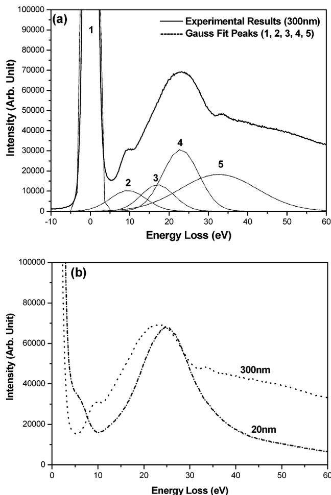
**Figure 3.** (a) Electron energy loss spectrum taken from Sb nanowire with diameter about 300 nm and its Gaussian-fit band with five peaks (1, 2, 3, 4, 5). (b) Series of electron energy loss spectra taken from Sb nanowires with nominal diameters of 300 and 20 nm.
