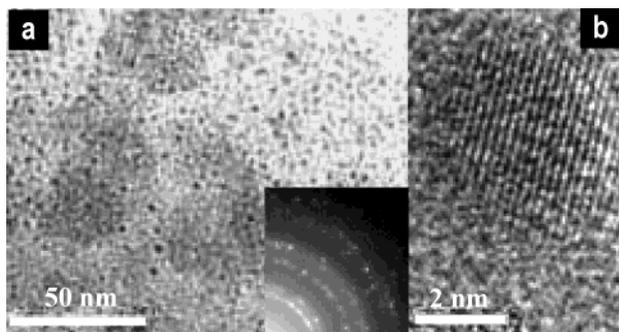
**Figure 1.** TEM images of Sb nanoparticles. (a) Low-magnification TEM image of Sb nanoparticles in starting solution. The inset shows the selected area electron diffraction pattern of these nanoparticles. (b) High-resolution TEM image of a 4 nm nanoparticle.
