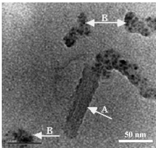
**Figure 4.** TEM image of intermediate state (by aging the starting solution for 4 days) of Sb nanoparticle–nanowire transition. Nanorod and nanorod-like structures of aggregated Sb nanoparticles are marked by A and B arrows, respectively.
